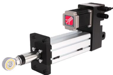
These actuators, which are applied during the reel unwinding and rewinding process, perform rapid and precise movements, thanks to the use of a recirculating ball screw. The available models allow stroke between +/- 25 mm and +/- 100 mm and a maximum thrust of 10000 N.
