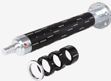
Re friction shafts are the ideal solution for multiple and independent rolls rewinding on the same shaft; their expanding rolls on friction rings guarantee a wide supporting surface. Air expanding shafts with rollers or with balls can be used with cardboard and plastic cores, ensuring no damages of the cores so that they can be reused several times. Friction rings can be equipped with preloaded positioners to center the reel core.
